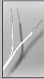
FIG. 3-6 Splitting and stripping.
